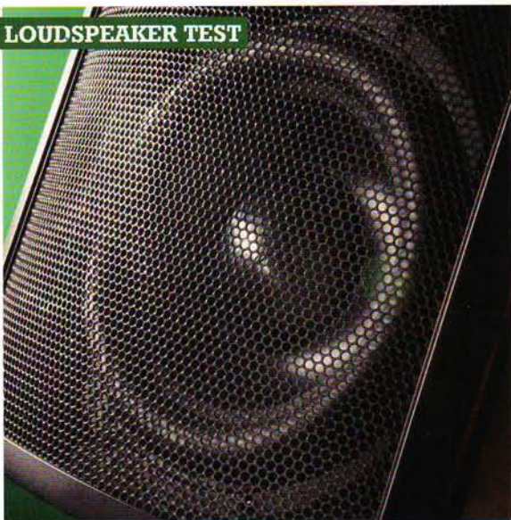
ABOVE: Bass frequencies are handled by this 10in driver, working into a sealed lower enclosure
